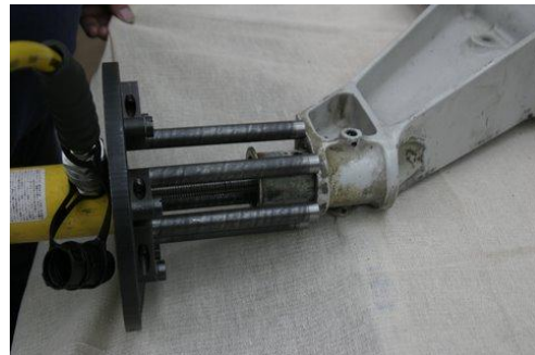
6 Operating the pump pulls out the bush
