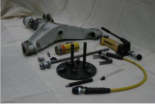
1 'BushOut' kit parts used to pull out the bush
