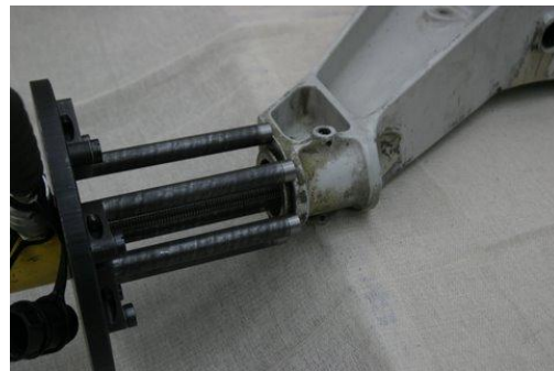
4 Assemble the tooling into the bush compressing the collet sliding it in until it expands locating the nibs behind the bush.
