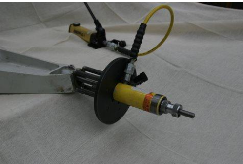
5 The removal assembly positioned ready to pull out the bush.
