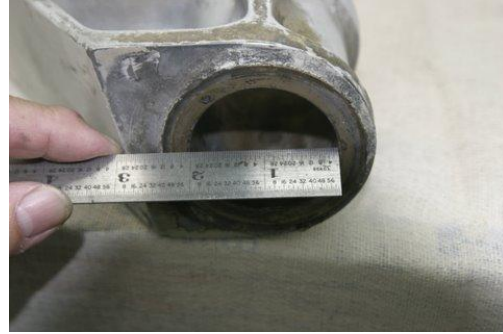
2 Measuring the internal bore of a bush.
